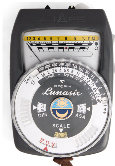
Figure 2: Gossen Lunasix — note the straight scale
